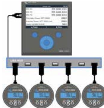
A maximum of four BMVs can be connected directly to a Color Control GX. Even more BMVs can be connected to a USB Hub for central monitoring.
