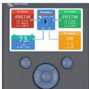
Color Control GX, showing a PV application
