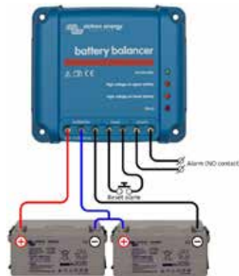
Battery Balancer (BMS012201000) The Battery Balancer equalizes the state of charge of two series connected 12V batteries, or of several parallel strings of series connected batteries. When the charge voltage of a 24V battery system increases to more than 27V, the Battery Balancer will turn on and compare the voltage over the two series connected batteries. The Battery Balancer will draw a current of up to 1A from the battery (or parallel connected batteries) with the highest voltage. The resulting charge current differential will ensure that all batteries will converge to the same state of charge.
