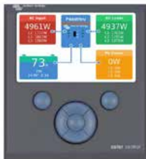
Color Control GX, showing a PV application
