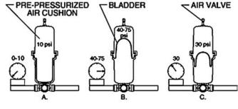
chamber forces water into the system. Pump stays off until minimum pressure is reached. Then pump turns on.
