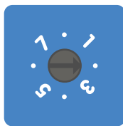
Rotary switch set to position 2
