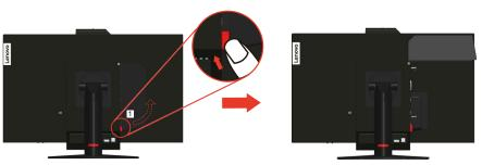
2. Pivot the rear Wi-Fi antenna downward at an angle of about 90°. Then, hold the thicker end of the rear Wi-Fi antenna and unscrew it from the computer.
