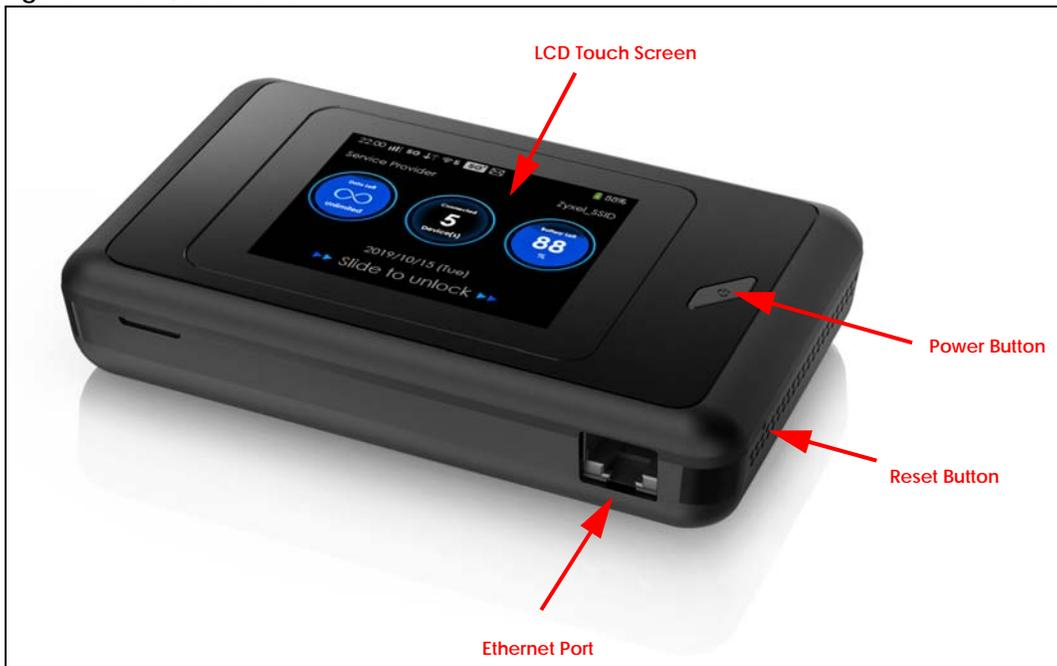
You can use Power Button on the front panel to turn on the NR2101 and use LCD Touch Screen to navigate the NR2101.
